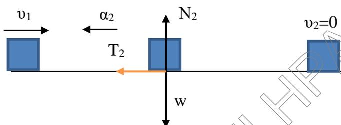
$$\Sigma F_y = 0 \Rightarrow N_2 - W = 0 \Rightarrow N_2 = 40 \text{ N και } T_2 = \mu N_2 \Rightarrow T_2 = 20 \text{ N}$$
